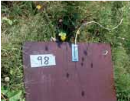
A Lufthansa Boeing 747-400 flies over the DLR's array of microphones (top); one of the 276 microphones used (bottom).
