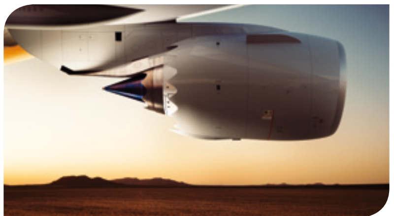
The newly developed GEnx-2B67 engines of the Boeing 747-8 are exceedingly fuel efficient and quiet.
