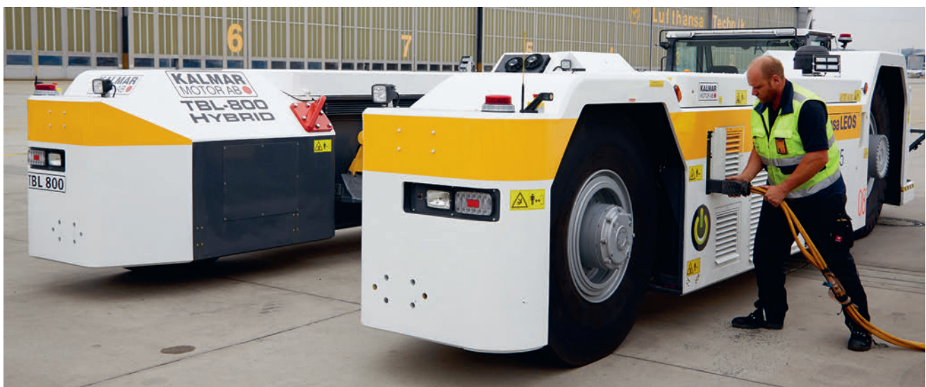
The eSchlepper diesel-electric hybrid aircraft tug is particularly suited for environmentally friendly maintenance and positioning tows of large passenger aircraft.
