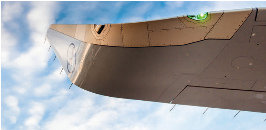
Especially impressive at a height of 2.4 meters, the wing-tip extensions or “sharklets” of the A320neo yield aerodynamic improvements and thus increase fuel efficiency.
