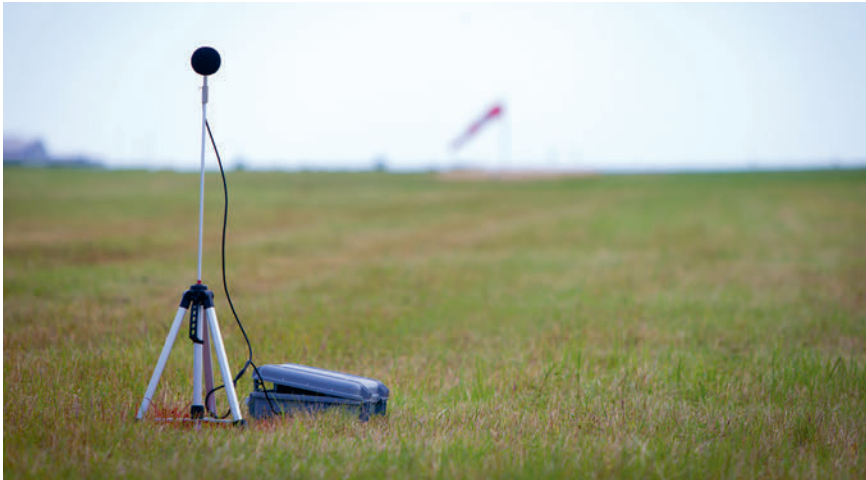
In 2015, flyover measurements were conducted at Magdeburg-Cochstedt Airport with Lufthansa Cargo MD-11 freight aircraft to test noise-reducing modifications on engines and landing gear.
